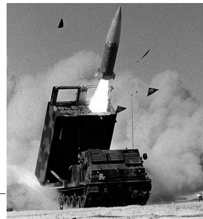
The MLRS systems fires a ATACMS Block 1 rocket composed of 950 sub-munitions (Lockheed Martin)
